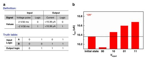
Fig. 7 Realization of the OR logic gate function with PFTPA-Fc memristor. a Definition for the logic inputs/outputs and truth table. b Experimental results of the PFTPA-Fc device
