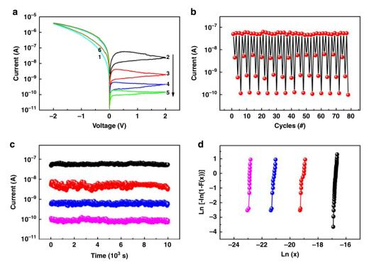
Fig. 4 Multilevel memristive switching characteristics in high resistance state. a Current-voltage curves of the ITO/PFTPA-Fc/Pt device. b Endurance and c retention performance of the multilevel storage. d Weibull distribution of the device current in the different conductance stages
