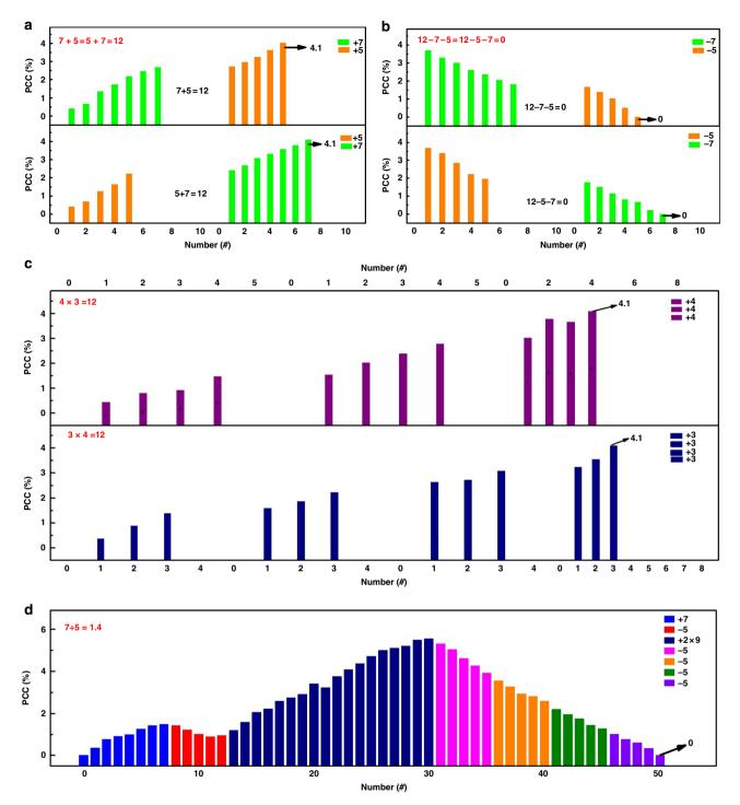
**Fig. 6** Demonstration of arithmetic computing with the PFTPA-Fc memristor. **a** Commutative addition, **b** subtraction, and **c** multiplication, as well as **d** fractional division conducted with the ITO/PFTPA-Fc/Pt device
