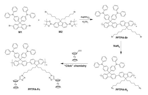
Fig. 1 Synthesis of the redox active polymer PFTPA-Fc
