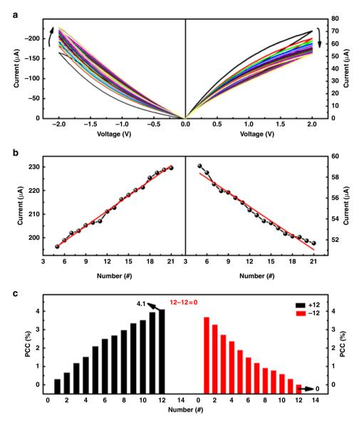
**Fig. 5** Consecutive memristive switching characteristics in low resistance state. **a** Current-voltage curves of the ITO/PFTPA-Fc/Pt device. **b** Linear relationship between the device currents read at  $\pm 2$  V and voltage sweeping numbers. **c** Calibration of the PFTPA-Fc memristor with the operation of 12–12 = 0 for decimal arithmetic calculations
