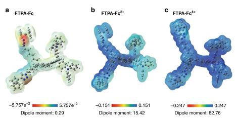
**Fig. 3** Electrostatic potential (ESP) distributions of the FTPA-Fc repeating unit. Simulated ESP profile in different oxidation states of **a** prinstine FTPA-Fc, **b** FTPA-Fc<sup>2+</sup>, and **c** FTPA-Fc<sup>4+</sup>, respectively. The gray, white, blue and light purple spheres represent carbon, hydrogen, nitrogen, and iron atoms, respectively
