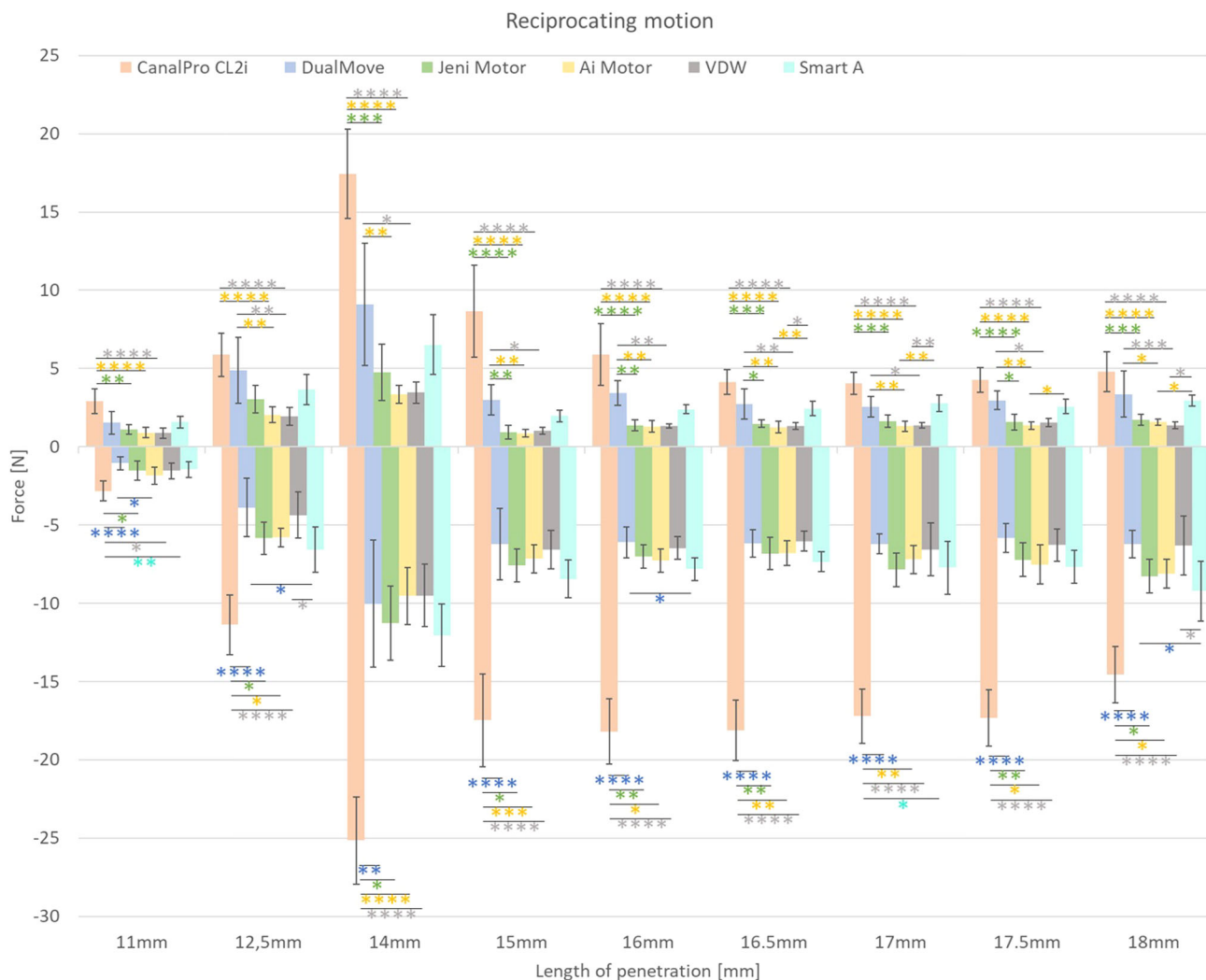
Fig. 4 P/R results after shaping of the resin blocks with One RECI instruments drove by different endodontic motors (* P > 0.05 ; ** P > 0.01 ; *** P > 0.001 ; **** P > 0.0001 ). The positive and negative forces represent the penetration and removal forces, respectively. When statistical significance is present, the statistical significance marks have the color of the best endodontic motor.
