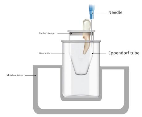
**Fig. 1** Schematic representation of the debris collection test model. The mesial root was inserted into a hole made on the stopper of an empty eppendorf tube. To keep the air pressure inside and outside of the tubes balanced, a 27-gauge bent needle was inserted. The whole apparatus was concealed in a glass vial covered with adhesive plaster to prevent the operator from seeing through during the instrumentation process. The whole assembly was mounted in a metal container.
