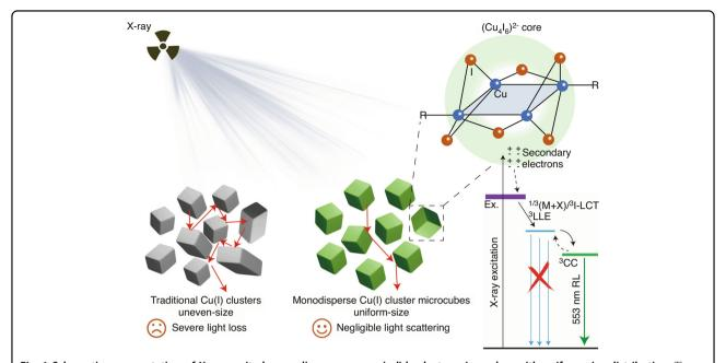
Fig. 1 Schematic representation of X-ray-excited monodisperse copper-iodide cluster microcubes with uniform size distribution. These microcubes emit 535 nm radioluminescence originating from triplet cluster-centered excited state (3CC) and show negligible light scattering
