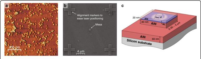
Fig. 13 Description of the sample structure. a  $1 \times 1 \, \mu m^2$  AFM image taken in height mode of the top plane of GaN QDs displaying a broad distribution of dot sizes. b  $26 \times 26 \, \mu m^2$  secondary electron image of the SA QD sample after evaporation of the top QD plane and etching into mesa structures. The displayed mesa is 1  $\mu$ m wide. c Sketch of the mesa structure. In practice, several QDs can be present on each mesa depending upon their dimension
