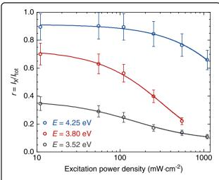
Fig. 10 Low temperature (T=5 K) evolution of the  $l_X/l_{\rm tot}$  ratio as a function of excitation power density for various QD emission energies. Solid lines serve as a guide to the eye
