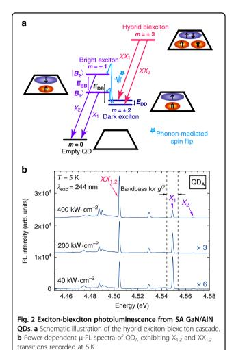
QDs remain efficient optical emitters up to RT with a large energy separation between confined energy levels.
