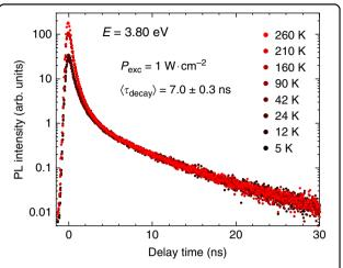
Fig. 9 Photoluminescence decays of GaN QDs emitting at 3.80 eV recorded from 5 to 260 K at an excitation power density of 1 W cm<sup>-2</sup>. All curves are stacked in order to superimpose the tail of the TRPL transients. The channel resolution was reduced down to 80 ps/channel to improve the qualitative appraisal of decay time conservation
