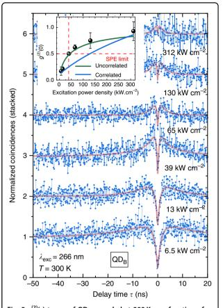
Fig. 5  $g^{(2)}(r)$  traces of QD<sub>B</sub> recorded at 300 K as a function of excitation power density with a channel resolution of 100 ps/ channel (blue connected diamonds) and convoluted fits (red lines). Inset: evolution of the single-photon purity with rising excitation power density where the solid lines are the results issued from models assuming either an uncorrelated background (green line) or a correlated one (blue line). Adapted from Tamariz et al.<sup>34</sup>
