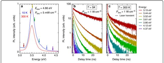
**Fig. 7 Time-resolved photoluminescence from a QD ensemble. a** Temperature dependence of the QD ensemble photoluminescence. The arrows mark the energies at which the TRPL transients shown in **b** and **c** are measured. The excitation power density is chosen low enough to ensure that most of the signal stems from excitonic recombination. Time-resolved photoluminescence transients measured at 5 K **b**. and 300 K **c**. are displayed. The laser transient is also given (grey line)
