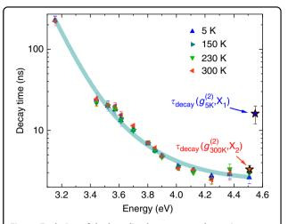
Fig. 11 Evolution of the long-lived component decay time  $\tau_L$  as a function of energy for temperatures ranging between 5 and 300 K. Decay times extracted from  $g^{(2)}(\tau)$  traces measured on QD<sub>A</sub> at 5 K and at RT are also reported for comparison (blue and red stars). The solid line serves as a guide to the eye
