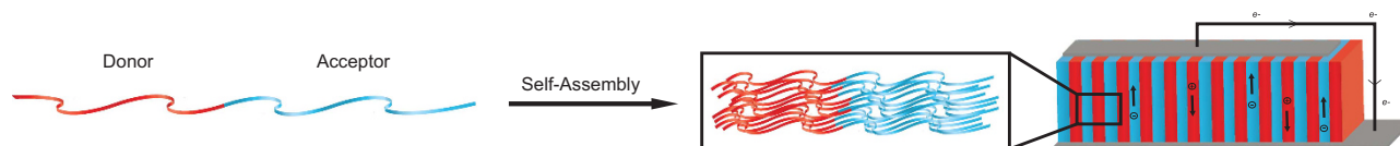
Figure 1 Schematic of proposed block copolymer self-assembly into lamellar active layer morphology.
