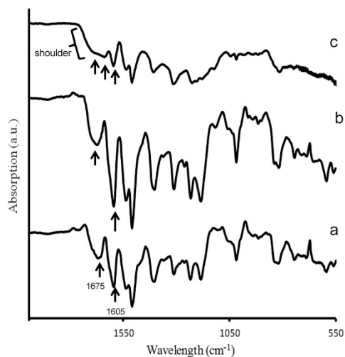
Figure 5 FT-IR spectra of PATAMDU films metal adsorbed by different methods: (a) pure films without any salts, (b) films made from the mixture of polymer with \text{Eu}(\text{NO}_3)_3 , (c) films swollen in \text{Eu}(\text{NO}_3)_3 solution.
