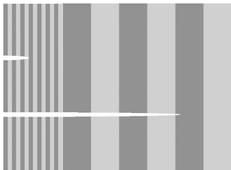
Figure 6 Double protection by the exocuticle with a small helical pitch and the endocuticle with a large helical pitch. The exocuticle protects the inside for small cracks with a small toughness, whereas the endocuticle protects the inside for large cracks with a large toughness.
