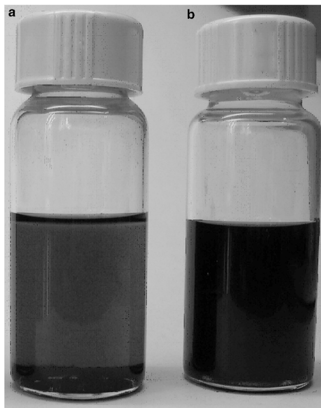
Figure 5 Stability of pristine SWNTs ( t = 1 h) (a) and PIp/SWNT composites (1.0 weight % SWNTs) ( t = 120 h) in \text{CHCl}_3 (after sonication for 60 min) (b). The SWNT content in each of the bottles was 0.2 mg/ml. A full color version of this figure is available at Polymer Journal online.
