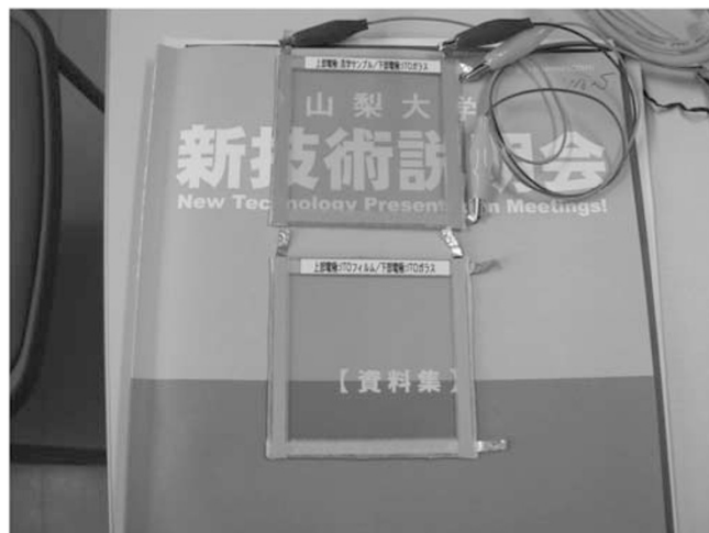
Figure 3 Prototype touch screens fabricated using a poly(3,4-ethylenedioxythiophene)/poly(4-styrenesulfonate)/polycarbonate (PEDOT/PSS/PC) film (top) and indium tin oxide (ITO) film (bottom), respectively. A full color version of this figure is available at Polymer Journal online.
