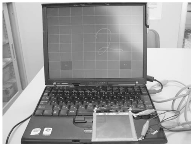
Figure 4 The number '2' on a polycarbonate (PC) screen written using a finger, or pen input by the touch screen fabricated using the poly(3,4-ethylenedioxythiophene)/poly(4-styrenesulfonate)/polycarbonate (PEDOT/PSS/PC) film as the top electrode. A full color version of this figure is available at Polymer Journal online.
