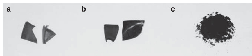
Figure 3 Photographs of as-formed free-standing P2Cz-D (a) and P(2Cz-D-co-EDOT) (2Cz-D:EDOT=1:5) (b) films and PEDOT powder (c) in the dedoped state electrosynthesized from \text{CH}_2\text{Cl}_2+0.1\text{-M Bu}_4\text{NBF}_4 .
