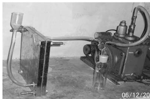
Figure 2 Vacuum-assisted resin transfer molding (VARTM) setup. A full color version of this figure is available at Polymer Journal online.
