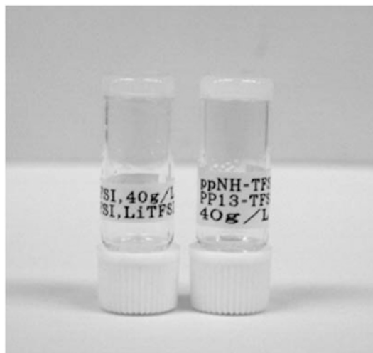
Figure 5 Ionogel of PP13-TFSA with 1 -TFSA at 40 g l -1 concentration (right) and ionogel of PP13-TFSA+10% LiTFSA with 1 -TFSA at 40 g l -1 concentration (left) in upturned vials.
