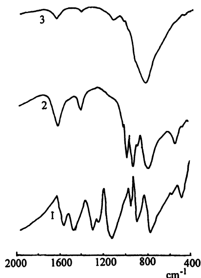
Figure 6. IR spectra of C_6H_{4.5}N(SiW_{11}V)_{0.106} treated by heating at different temperature. 1, 210°C; 2, 450°C; 3, 620°C.
