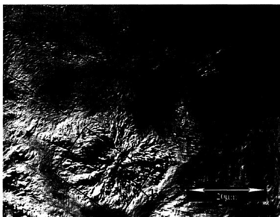
Figure 2. CLSM image of the same area of a sample as Figure 1. A and B are PBSU and P(VDC-VC) spherulites, respectively.
