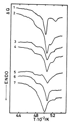
Figure 7. DSC curves of the CA(2.46) fractions (1--6) and a whole polymer (7) at a heating rate of 10 K/min. 1,  $M_w = 5.3 \times 10^4$ ; 2,  $M_w = 7.4 \times 10^4$ ; 3,  $M_w = 1.08 \times 10^5$ ; 4,  $M_w = 1.41 \times 10^5$ ; 5,  $M_w = 1.85 \times 10^5$ ; 6,  $M_w = 2.65 \times 10^5$ ; 7,  $M_w = 1.2 \times 10^5$ .
