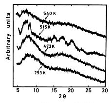
**Figure 11.** X-Ray diffractograms of the CA(2.46) fraction (EF3-14) at temperatures from 293 to 540 K. Curve numbers denote temperature.
