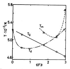
**Figure 14.** Total degree of substitution  $\langle\!\langle F \rangle\!\rangle$  dependence of  $T_g$ ,  $T_m$ , determined by DSC and  $T_d$  by TG.  $\bigcirc$ ,  $T_g$ ;  $\triangle$ ,  $T_m$ ;  $\square$ ,  $T_d$ . Solid line,  $T_g$ ; broken line  $T_m$ ; chain line,  $T_d$ .
