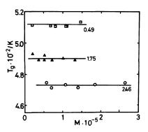
**Figure 10.**  $T_g$  of CA(2.46), CA(1.75) and CA(0.49) fractions determined by DSC as a function of molecular weight.  $\bigcirc$ , CA(2.46);  $\triangle$ , CA(1.75);  $\square$ , CA(0.49). Numbers on the lines denote total degrees of substitution.
