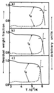
**Figure 12.** Thermogravimetry (TG) and differential thermogravimetry (DTG) curves of the CA(2.92) ( $M_w = 1.49 \times 10^5$ ), CA(2.46) ( $M_w = 1.41 \times 10^5$ ) and CA(0.49) ( $M_w = 1.45 \times 10^5$ ) fractions. Solid line, TG curve; broken line, DTG curve.  $T_d$ , temperature at start of decomposition.
