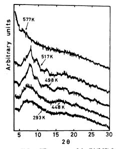
**Figure 5.** X-Ray diffractograms of the CA(2.92) fraction (TA3-4) at temperatures from 293 to 577 K,  $2\theta$ , diffraction angle. Number to each curve denotes temperature.
