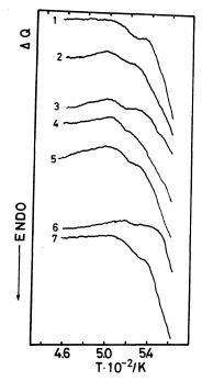
Figure 9. DSC curves of the CA(0.49) fractions (1-6) and a whole polymer (7) at a heating rate of 10 K min<sup>-1</sup>. 1,  $M_w = 4.55 \times 10^4$ ; 2,  $M_w = 6.76 \times 10^4$ ; 3,  $M_w = 7.94 \times 10^4$ ; 4,  $M_w = 1.08 \times 10^5$ ; 5,  $M_w = 1.11 \times 10^5$ ; 6,  $M_w = 1.45 \times 10^5$ .
