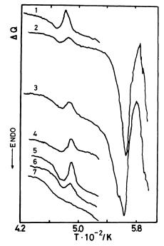
Figure 1. Differential scanning calorimetry (DSC) curves of CA(2.92) fractions (1-6) and a whole polymer (7) at the heating rate 10 K min<sup>-1</sup>. 1, viscosity-average molecular weight  $M_v = 4.7 \times 10^4$ ; 2,  $M_v = 1.97 \times 10^5$ ; 3,  $M_v = 2.22 \times 10^5$ ; 4,  $M_v = 3.59 \times 10^5$ ; 5,  $M_v = 4.56 \times 10^5$ ; 6,  $M_v = 5.83 \times 10^5$ ; 7, weight-average molecular weight  $M_w = 2.35 \times 10^5$ .
