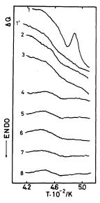
Figure 4. DSC curves of the CA(2.92) fraction (TA3-4) with  $M_v = 2.22 \times 10^5$  at a heating rate 10 K min<sup>-1</sup>. 1, curves in heating process; 1', cooling immediately after heating (curve 1); 2–8, repeating order of cycle and curves during heating.
