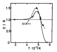
Figure 6. Relation between diffraction intensity ratio (DIR) estimated from the X-ray diffractograms of CA(2.92) and CA(2.46) and temperature.  $-\bigcirc$ , CA(2.92) fraction, ---, CA(2.46) fraction.
