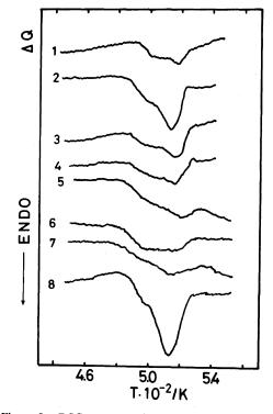
Figure 8. DSC curves of the CA(1.75) fractions (1-7) and a whole polymer (8) at a heating rate of 10 K min<sup>-1</sup>. 1,  $M_v = 2.1 \times 10^4$ ; 2,  $M_w = 3.75 \times 10^4$ ; 3,  $M_v = 5.53 \times 10^4$ ; 4,  $M_w = 5.54 \times 10^4$ ; 5,  $M_v = 7.72 \times 10^4$ ; 6,  $M_w = 1.00 \times 10^5$ ; 7,  $M_w = 1.31 \times 10^5$ .
