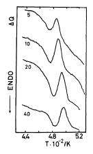
Figure 3. DSC curves of CA(2.92) fraction (TA3-4) with  $M_v = 2.22 \times 10^5$  at a heating rate from 5 to 40 K min<sup>-1</sup>. Number on each curve denotes heating rate.
