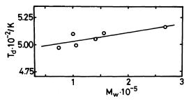
**Figure 13.**  $T_{\rm d}$  of CA(2.46) fractions determined by TG as a function of weight-average molecular weight  $M_{w}$ .
