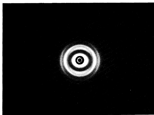
Figure 7. \beta Poly(L-isoleucine): The X-ray diffraction photograph. (Cylindrical camera, Cu-K \alpha radiation) Fiber axis, vertical).
