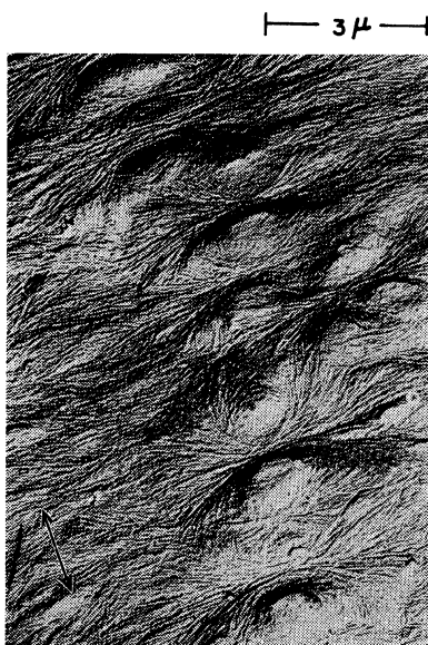
Figure 1. Typical electron micrograph of free specimen surfaces. Arrow indicates the extrusion direction.
