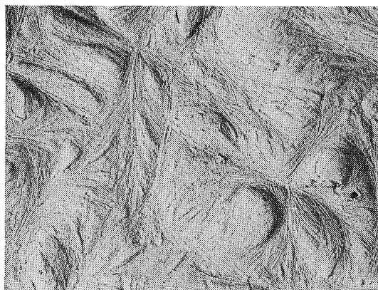
Figure 8. The electron micrograph of the poly(chlorotrifluoroethylene) film which gave rise to the scattering patterns shown in Figure 5.
