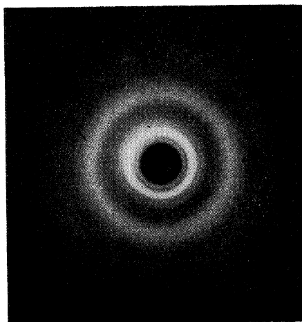
Figure 4. X-ray diffraction pattern of the stereocomplex obtained from the 1:2 (iso/synd) mixture in acetone.
