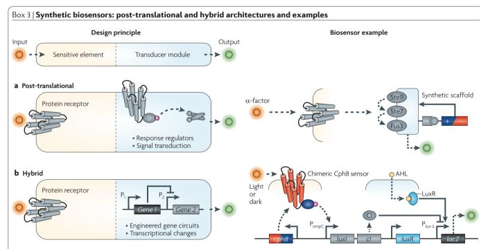
A basic biosensor has two modules (see the figure): the sensitive element recognizes and binds analytes, whereas the transducer module transmits and reports signals.
