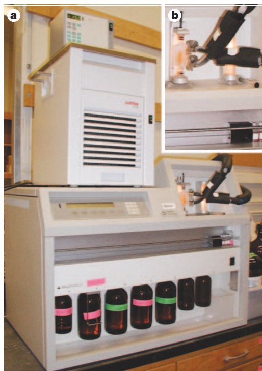
Figure 2 | The first automated oligosaccharide synthesizer. Device (a) is based on a modified peptide synthesizer. The reaction vessel (b) is shown in the inset.
