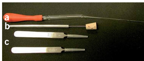
Figure 2 | Tools for manipulating oocytes. (a) Fine glass pipette prepared from a Pasteur pipette drawn out over a Bunsen flame, (b) dissecting needle and (c) Dumont forceps no. 5 (Dumostar).
