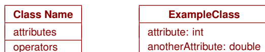
Figure 1: (Left) The general form of a UML class diagram. (Right) Example of a class diagram of the sort seen in SBML. SBML classes never use operators, so SBML class diagrams only show the top two parts.
