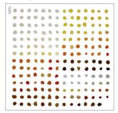
How many scientists would love to have a small and cheap spectrometer? Jie Bao and Moungi Bawendi have come up with a solution by integrating almost two-hundred absorptive filter arrays made of colloidal quantum dots and a charge-coupled device detector into a coin-sized digital camera capable of resolving spectral peaks separated by mere nanometres. Such resolution and compactness may find applications in medicine or space exploration.
