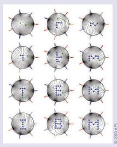
the chamber into position. By controlling individually the rate of flow in or out of each inlet or outlet, the shape of these fields can be intricately controlled. This in turn can be used to guide the flow of suspended particles, and, by using particles that stick together when they come into contact, could be used to guide the formation of complex structures.
