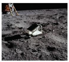
One of the scientific milestones of the Apollo 11 mission to the Moon was the installation of an optical retroreflector array (pictured) on the lunar surface. Its 100 fused-silica cubes reflect laser pulses sent from Earth; from the delay of the return signal, the Moon–Earth distance can be determined with a precision of a couple of centimetres.
