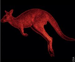
a diffraction efficiency over 99% at a 1600 nm wavelength," say the authors of the paper. "This is the highest efficiency of any metahologram demonstrated to date reproducing grayscale images over a broad spectral range." In this context, diffraction efficiency is defined as the power in the holographic image with respect to the total power transmitted by the metahologram.
