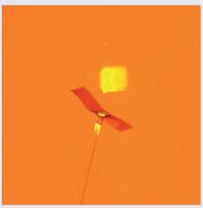
The size of the gripping force is proportional to the excitation light intensity, and for a light level of 100 mW cm<sup>-2</sup>, the force was 250  $\mu$ N, which is sufficient to sustain an object with a weight of tens of milligrams. The gripper rapidly releases the object once the light is turned off. The response time of the light-driven flytrap also depends on the light power, with the gripper closing within 200 ms for light power of about 300 mW.
