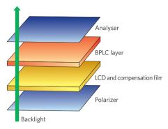
A new method of controlling the viewing angle of a liquid-crystal display (LCD) promises greater privacy to users of mobile phones and laptops. By inserting a bluephase liquid-crystal (BPLC) layer into an LCD, Shin-Tson Wu and colleagues from the University of Central Florida, USA, were able to tune the viewing angle of the display continuously when adjusting an applied voltage.
