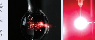
of 1 kHz, pulse energy of 1 mJ and beam diameter of 7 mm) onto a droplet of distilled water. The peak power of the laser pulses was varied over the range of 1-25 GW. The droplet emission was measured by a spectrometer in the wavelength range of 195-1,150 nm.
