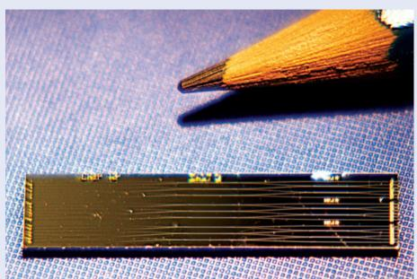
algorithm, then outputs the answer — 3 and 5," O'Brien told *Nature Photonics*. "On the chip the photons travelled through silica waveguides that were brought together to form a sequence of quantum logic gates, and the output was determined by which waveguides the photons exited the chip from."
