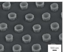
Octopus arms can adhere to various surfaces in marine environments because of their periodic, non-close-packed, centimetre-scale suckers. However, existing octopus-inspired artificial suckers still suffer from reliance on suctioning systems and power sources or poor applicability to rough surfaces and wet environments. Ying-Chu Chen and Hongta Yang now report the assembly of nanosucker adhesive arrays, capable of adhering to both microrough and flat surfaces in dry and wet environments.
