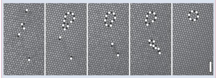
Visualizing the diffusion of dislocations in a crystal can provide important insights into the mechanical properties of the material. Ossi Lehtinen and colleagues at the University of Ulm, the University of Helsinki and Aalto University have now followed the full life cycle of dislocations in graphene, from creation to annihilation, with atomic resolution (*Nature Commun.* **4**, 2098; 2013).
