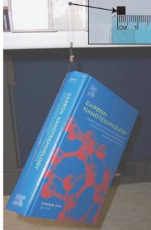
*Science* **322**, 238–242 (2008) Gecko lizards seem to defy gravity by climbing vertical surfaces. Only recently it was discovered that geckos acquire their sticking ability from microscopic hairs, called setae, on their feet. Now scientists in the US have made a material with ten times the adhesive strength of gecko feet, by using carbon nanotubes to mimic the setae structure.
