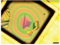
*Appl. Phys. Lett.* **92**, 123110 (2008) Potential applications of graphene — a single layer of carbon atoms — in nanoelectronics are limited by the lack of simple procedures for producing freestanding membranes and fabricating nanoscale structures on them. Now Jannik Meyer and colleagues at Berkeley have developed a straightforward way to overcome these problems by using electron beam induced deposition (EBID) of carbon to fabricate periodic patterns on freestanding graphene.
