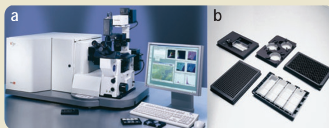
Figure 1 | The iCys research imaging cytometer. (a,b) The iCys instrument (a) and a sampling of the carrier types that can be analyzed on the system (b).
