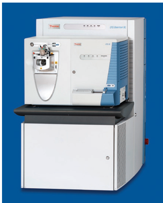
The LTQ-Orbitrap is an example of the trend for hybrid mass spectrometers. (Courtesy of Thermo Electron.)
