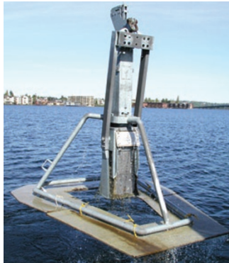
The coring device used for collecting undisturbed samples of the sediment in Lake Washington. Image courtesy of Mila Chistoserdova.
