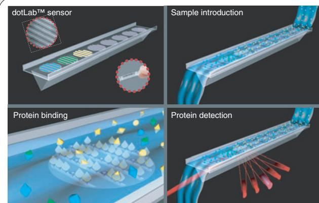
**Figure 1 |** dotLab basics. Capture molecules are deposited onto the sensor surface as a diffraction grating. Eight individual spots can be patterned in this fashion. Test solutions are introduced into the sensor, and as analytes bind on the surface, the efficiency of the diffraction grating improves. As the grating is interrogated during the binding reaction, an increase in diffraction signal is measured in real time.
