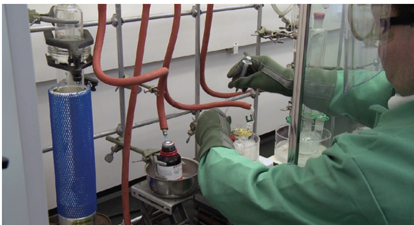
Researchers transfer an organolithium compound from a reagent bottle to a graduated funnel with a cannula (top) and to a reaction vessel with a syringe (bottom), avoiding exposing the chemical to air.
