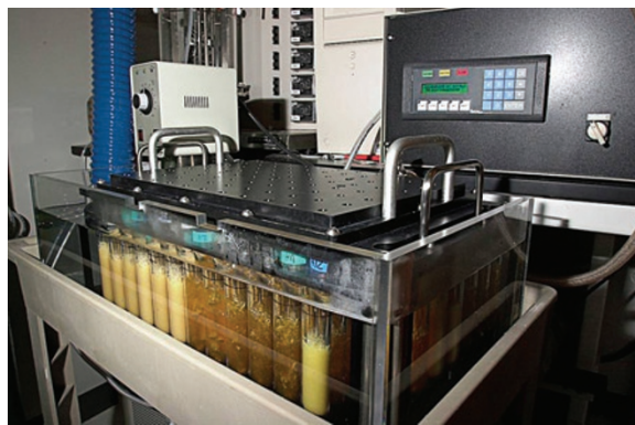
The GNF developed high-throughput bacteria fermentation system used by JCSG for large-scale protein production. (Courtesy of JCSG.)
