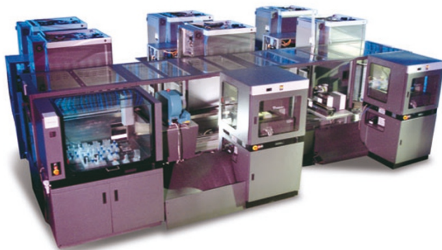
The CrystalMaker provides start-to-finish automation for protein crystallography. (Courtesy of Rigaku.)
