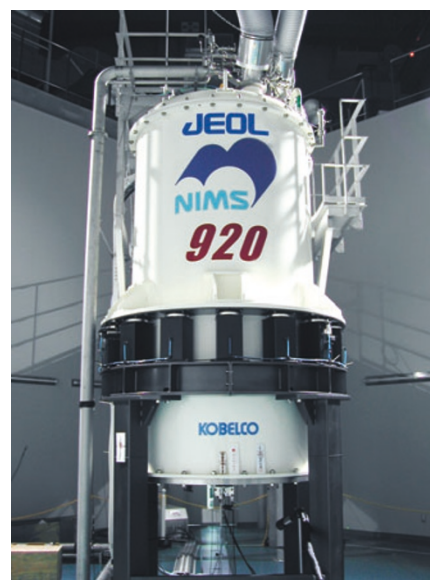
The ECA NMR system from JEOL can currently be configured with field strength of up to 920 megahertz. (Courtesy of JEOL USA.)
