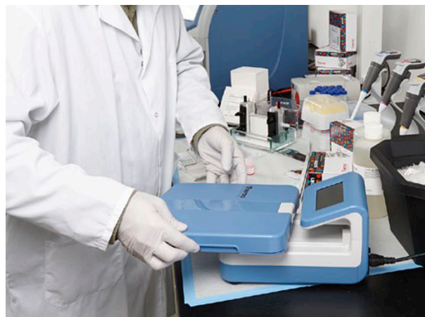
Figure 2 | The Pierce™ G2 Blotter cassette, which contains the gel, blotting membrane and filter paper, inserts easily into the power supply. The transfer conditions are then selected using the touchscreen panel on the unit.
