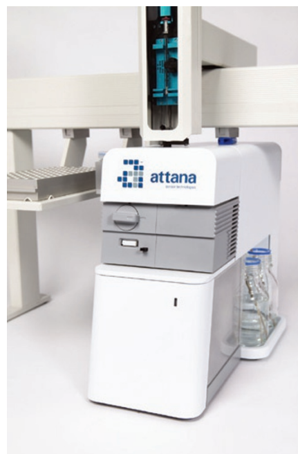
Figure 1 | The Attana A100, shown attached to a C-fast pipetting robot for automation.
