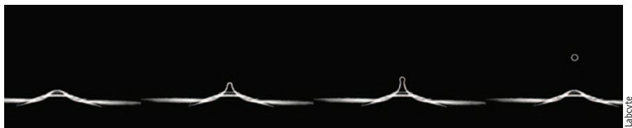
Labcyte's acoustic dispenser ejects a droplet from the fluid surface.
