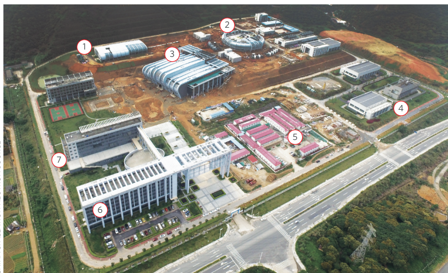
Figure 1 | Aerial photo of the China Spallation Neutron Source taken in April 2016. The facility is intended to be open for users from 2018. Numbering indicates the following: (1) linear accelerator (the actual accelerator is underground); (2) rapid cycling synchrotron; (3) the first target building and experimental hall; (4) main substation; (5) future site of the second target station; (6) offices and laboratories; (7) service building.
