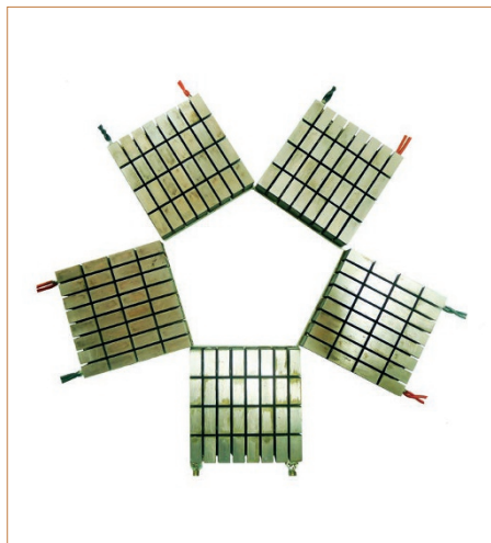
Figure 1 | Skutterudite-based thermoelectric modules manufactured by the Shanghai Institute of Ceramics, Chinese Academy of Sciences. Each module has dimensions of 50 mm × 50 mm, and a maximum output of 25 W for a 500 K temperature gradient.
