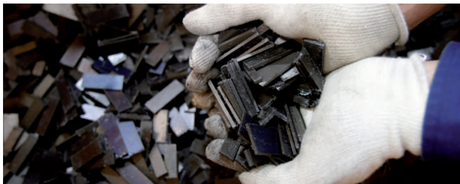
Rare-earth magnets being recycled at Hitachi.
