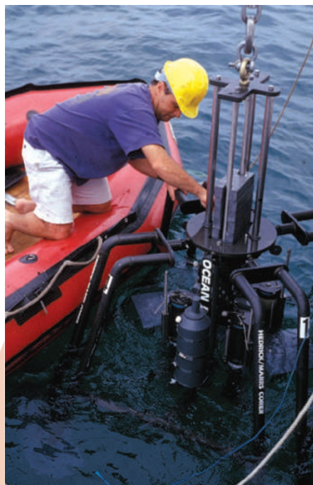
Peter Swarzenski setting up a multicorer at Lake Tanganyika, East Africa, to collect sediment cores to document the lake's climate and environmental history.
