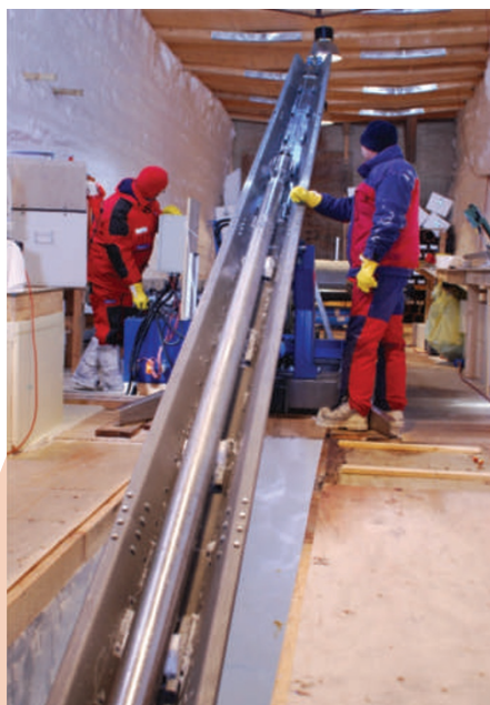
The drilling system at Talos Dome, where the TALDICE team extracted a palaeoclimate record of 1,620 m of ice.
